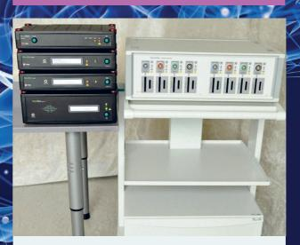
Tesla station brings easily movable trolley, built in battery (110 Ah) and a 320 channels system with color coded cap connectors into one package.
