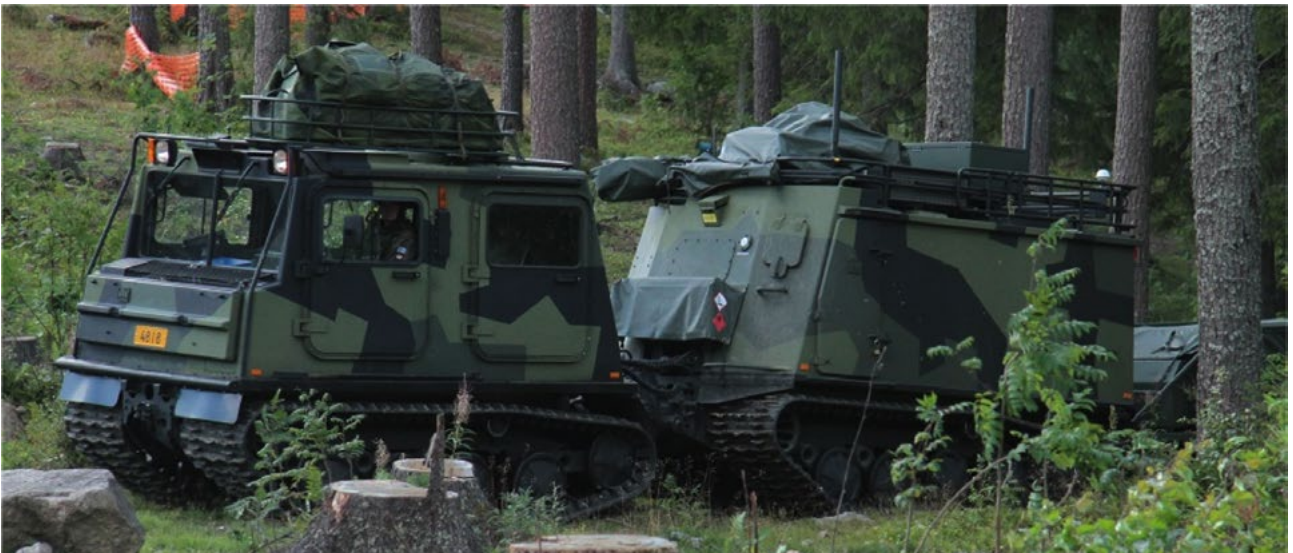
Figure 10: FDF Army signal vehicle on the move in the Finnish forest. With its MANET capability Bittium TAC WIN allows maintaining the access to the tactical IP network also while moving. The NATO band I (225 – 400MHz) antennas connected to the Bittium TAC WIN Radio Head I shown on the roof of the rear wagon. (Photo copyright: FDF).
