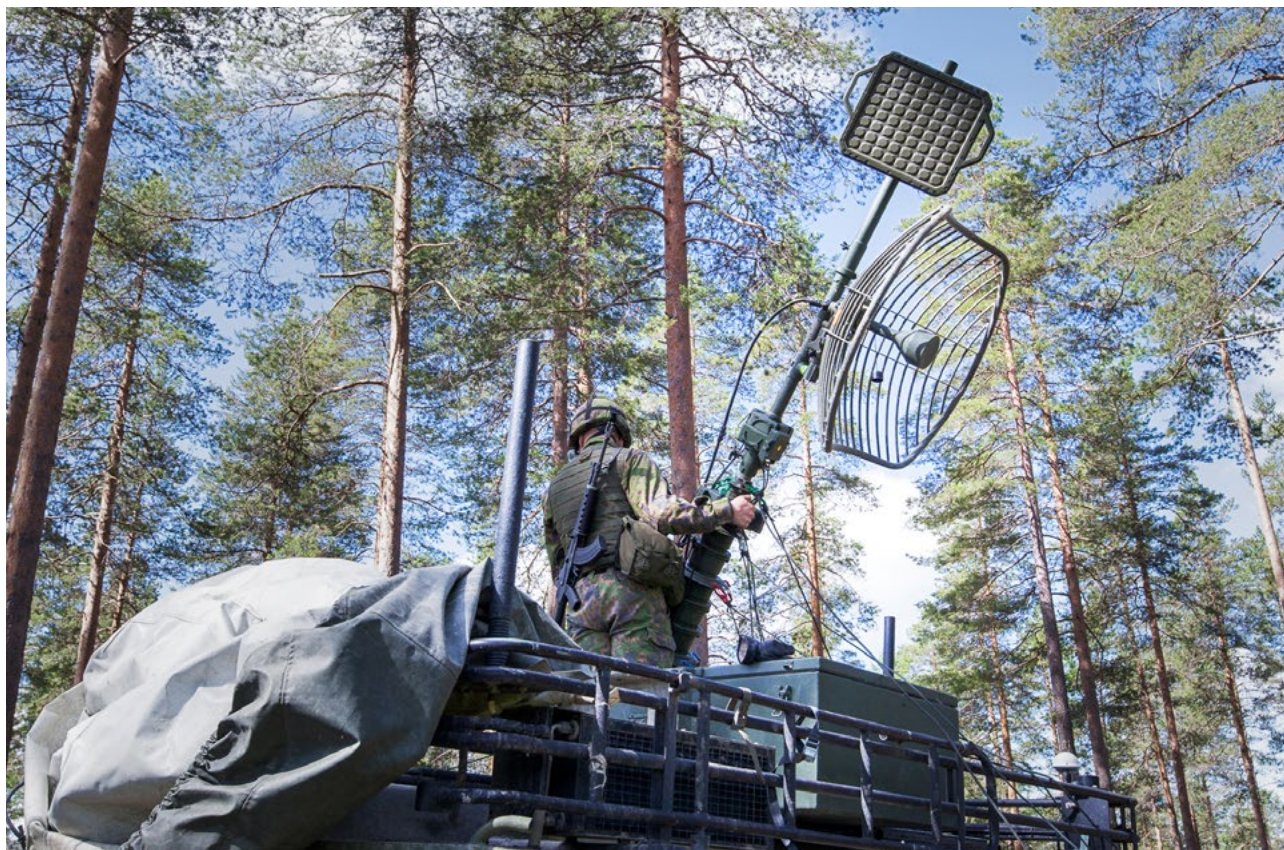
Figure 9: Setting up the NATO band III antenna and Bittium TAC WIN Radio Head IV with integrated NATO band IV antenna.
