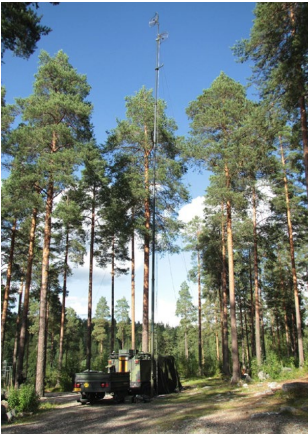
Figure 5: FDF Army signal vehicle. Bittium TAC WIN Radio Head III connected to NATO band III antennas shown on the top of the mast (Photo copyright: FDF)
