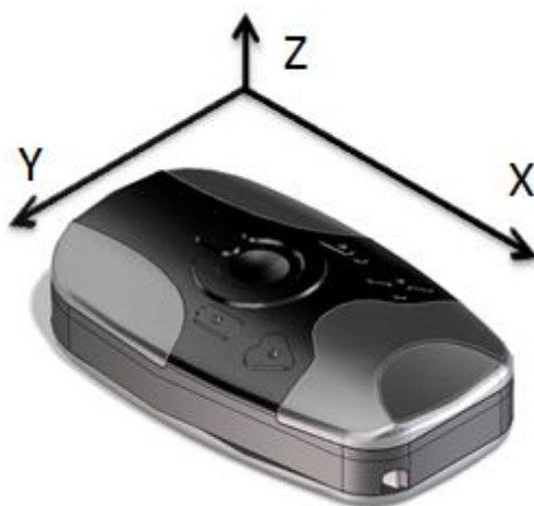
Figure 13 Accelerometer axis directions
