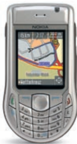
3SOFT GmbH's smartphone-based off-board navigation system guides the user with voice output and route shown on display.
